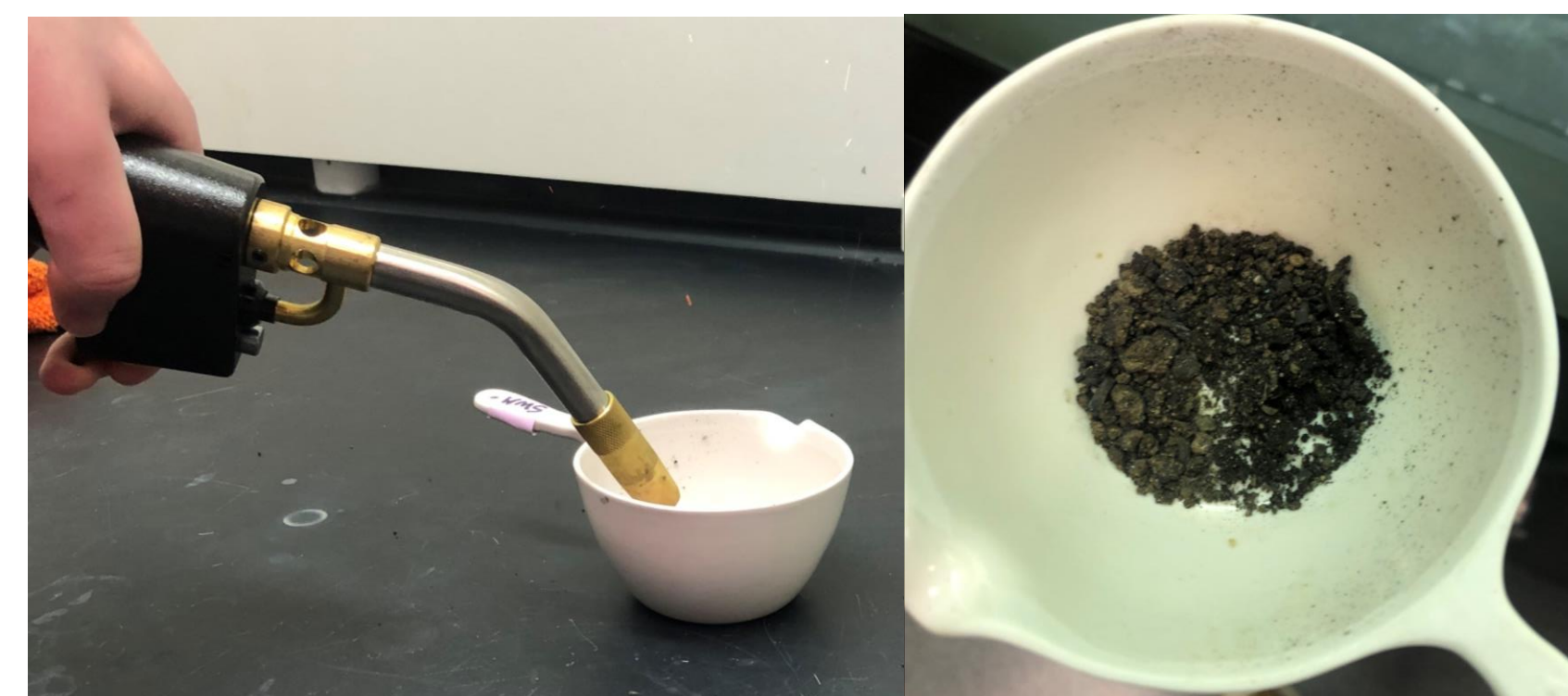
Figure 2. (Left) Lab Technician Bethany Tegt burning the Whatcom Middle School soil sample with a butane torch. (Right) Burnt soil sample contained in crucible.
