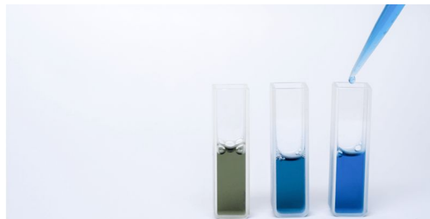
Figure 2. This picture shows how the Bradford Assay solution turns blue over time as the protein is added
