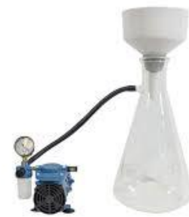
Figure 1: Buchner funnel pressurizes and funnels the solution through a filter.
