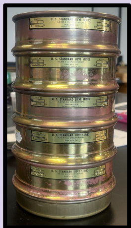
Figure (b): Sieve used to measure separating sand size.
