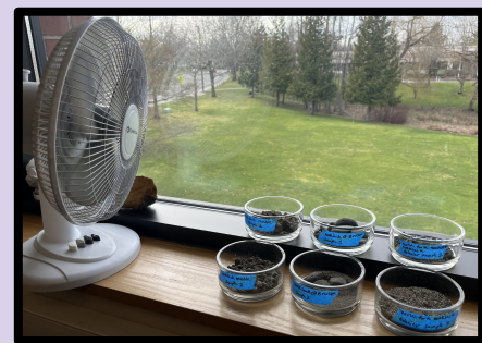
Figure (a): Sand samples being dried before being usable.
