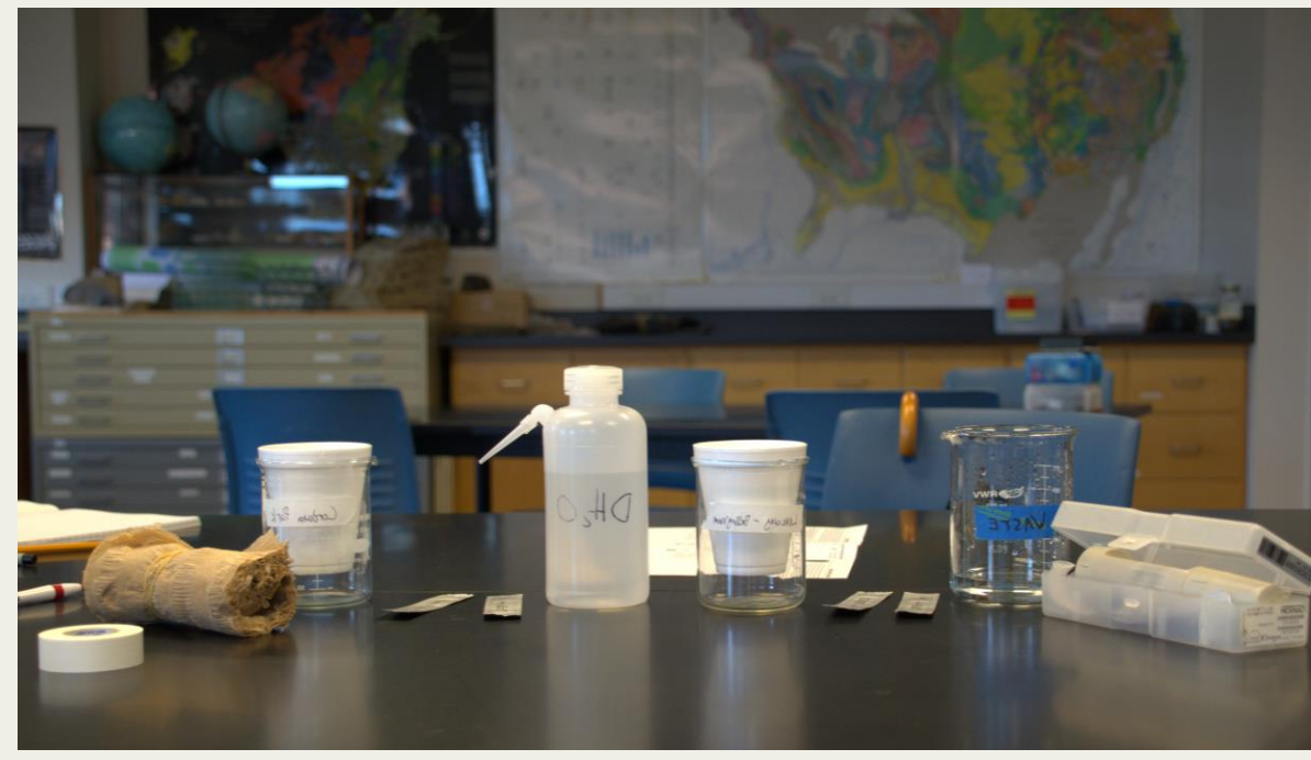
Figure 1. Materials used in experiment: x2 Styrofoam cups; x2 glass beakers; Eutech PCTest35 Probe Oakton, serial no. 2309389; LABTECH H2O OK Drinking Water Analysis Test Kit; Distilled water; masking tape; 'Low-cost Water Monitoring' tablet, by LaMotte
