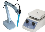
Figure 1. The instrument on the left is a pH meter probe. The instrument on the right is a continuous magnetic stirrer
