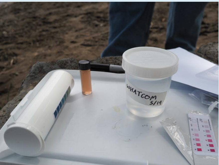
Fig. 2B: Water sample & dissolved oxygen vial at Lake Whatcom
